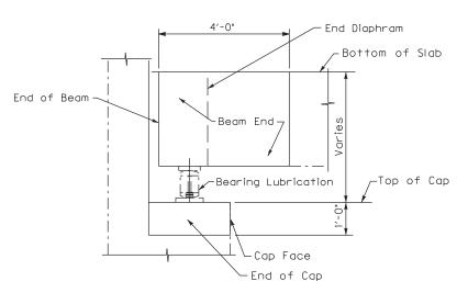
Front Face of End Wall, Top and Face of Cap the Entire Length of Cap including Cap Ends, Beam Ends and End Diaphrams shall have debris removed pressure washed and have concrete coating applied as specified within the limits shown.
